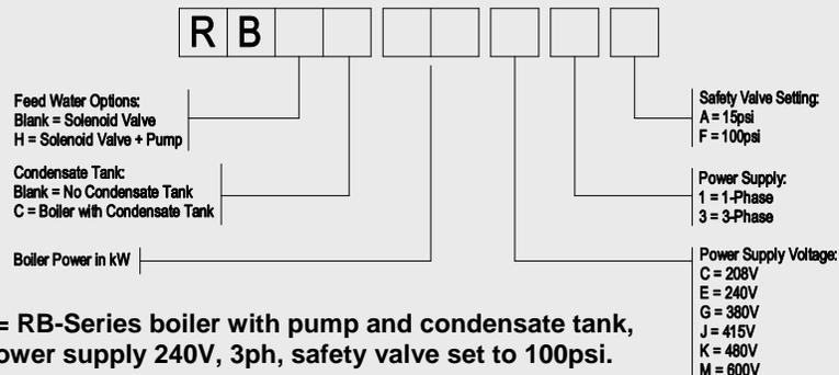
**Example:** RBHC20E3F = RB-Series boiler with pump and condensate tank, 20kW heating power, power supply 240V, 3ph, safety valve set to 100psi.
